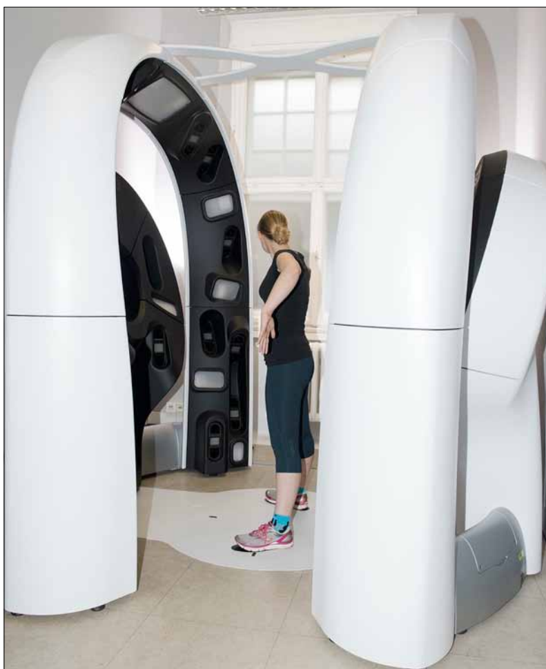
Fig. 2: Preoperative full body 3D-analysis is performed using the VECTRA WB360 (Canfield Scientific) imaging system. 3D-technology allows surgeons to model and plan surgery and to objectively analyze surgical outcome.
