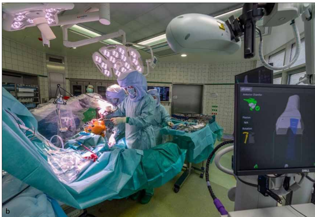
Fig. 1a, b: The MAKO consists of a camera system, a workstation and a robotic arm [1a © Stryker Orthopedics]
